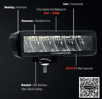
LMD-WL-618 1 lux @ 145m | Raw Lumens: 2.000 lm | Wattage: 18W | Voltage: 10-30V Housing: Aluminum | Lens: Polycarbonate | Weight: 0.62 kg | IP Rating: IP67-IP69k E-MARK Approved: ECE R10
